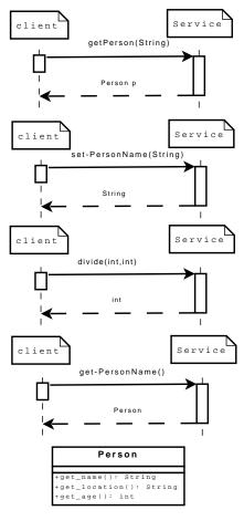
Fig. 1. Web service UML specification
