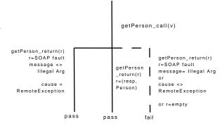
Fig. 12. Test cases generated from the "getPerson" operation
